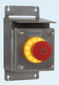
PSN\*NZ0762 Enclosed - Twist to release e-stop with mechanical eye indicator & 24V AC/DC luminous ring, 1 x self-monitoring contact & 1 x N/C contact block IP66/67 304 SS enclosure with sloping lid and mounting feet
